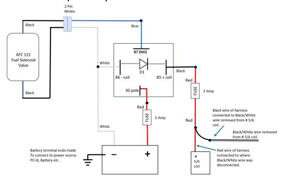
We are using the "safety circuit" 12 V Coil Black/White wire connection to trigger the relay. When the key is turned on, if the safety circuit is satisfied, 12 V is supplied to 85 of the relay, which energizes the relay. The relay then routes power from the battery through 30, to 87 of the relay, and energizes the fuel solenoid. The fuel solenoid will remain energized until any shutoff signal is received. The safety shutoff signals such as the
