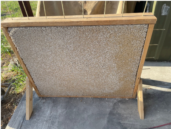
Custom Hempcrete Panel incorporating TREBAR to be precast either onsite or delivered from our facility to a company looking to add plant-based building materials into their portfolio.
