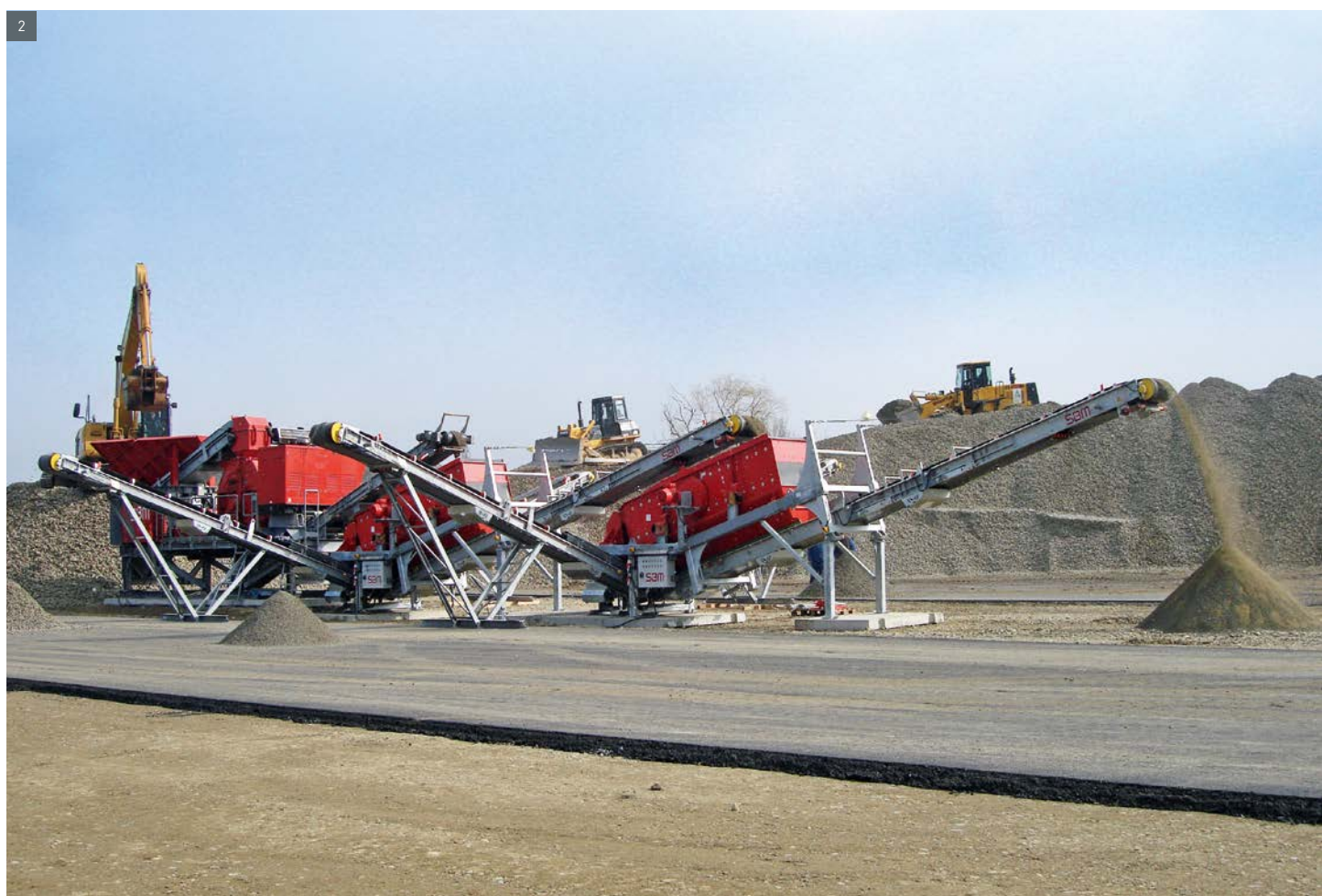
2. SMR 10/5/4 SEMI con dos tamices KQ 15/40-2 SEMI / SMR 10/5/4 SEMI with two screens KQ 15/40-2 SEMI
