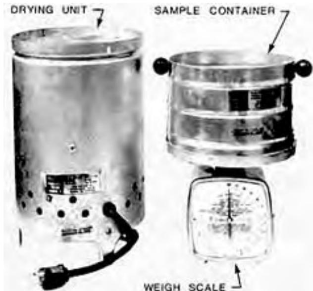
FIGURE 1. Koster Forage Moisture Tester.
