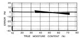
Accurate readings occurred at about 45% moisture content. FIGURE 3. Accuracy in Chopped Corn.
