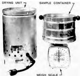
FIGURE 1. Koster Forage Moisture Tester.
