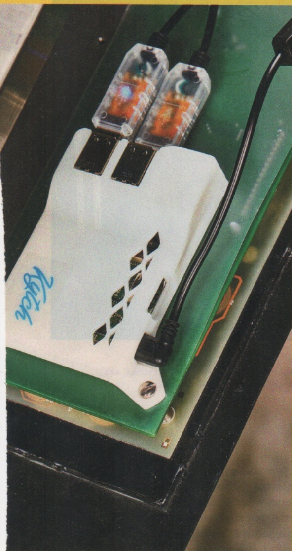
Kytch's device, built around a Raspberry Pi minicomputer, is designed to be installed inside a Taylor ice cream machine.
