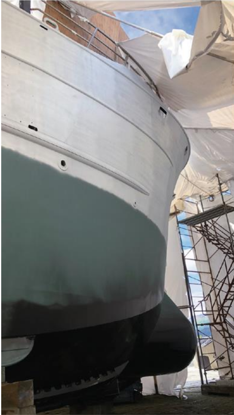
Fig. 2. These photos depict some of the marine structures that have recently been metalized by the fabricator, including (clockwise from left) ship hulls, rudders and metal stairways and railings.
