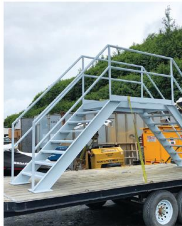
Fig. 2. These photos depict some of the marine structures that have recently been metalized by the fabricator, including (clockwise from left) ship hulls, rudders and metal stairways and railings.
