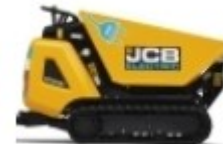
CONCRETE BUGGY, TRACKS
