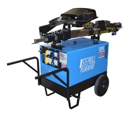
• The mast system folds down and securely locks for easy transport.
