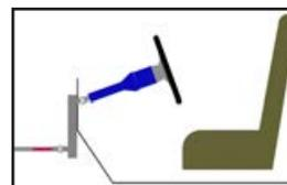
Adding the Steer Clear unit allows the column to stop at the firewall and allows the output shaft to be offset, positioning it lower in order to clear the engine.
