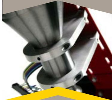
Attach the column to the mount using two steering column drops. Holes have been provided on the underdash mount to allow you to adjust the position of the column drops to where you see fit. The bigger the difference in length between the two drops, the greater the angle of the column will be.
