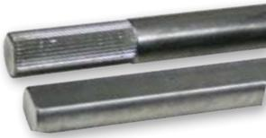
THIS MILD STEEL SHAFT IS CUT TO LENGTH AND INSTALLED IN THE RAG JOINT AND/OR U-JOINT. SET SCREWS LOCK IT IN PLACE. THE 3/4" DD SHAPE OFFERS A SAFE & INEXPENSIVE WAY TO REPLACE YOUR OLD SHAFT. COLLAPSIBLE SHAFTS ARE AVAILABLE, ASK YOUR SALES REPRESENTATIVE FOR DETAILS
