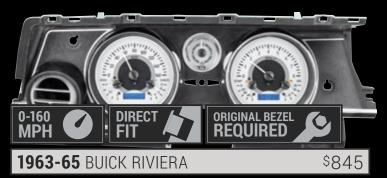
Fitting into your existing gauge bezel, your 1963-65 Riviera never had it so good! The inside of the original gauge pods must be clearanced slightly to install the new instruments, but the original gauge trim rings are reused! An analog clock is located in the center opening, with the six analog gauge readings and dual LCD message centers taking up residence in the large openings. Stock turn signal and high beam indicators are retained, but upgraded with LED illumination!
