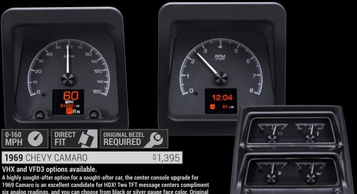
right canaro is an excellent candidate for HDX! Two TFT message centers compliment six analog readings, and you can choose from black or silver gauge face color. Original instrument lenses and indicator strips are eliminated with our billet aluminum, black powder coated trim rings. Main and satellite instruments fit into existing plastic bezels/ housings; main bezel sold separately. Center console instruments are part of the main system and cannot be used stand-alone.
