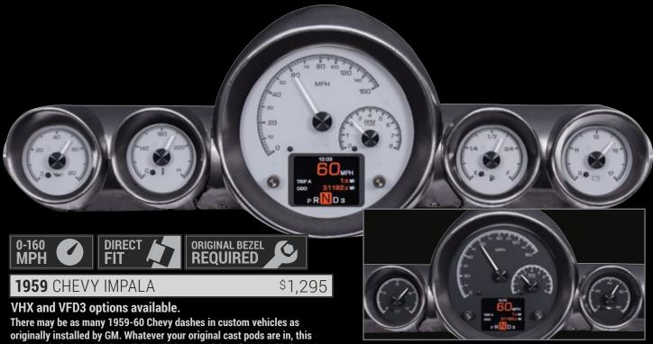
originally installed by GM. Whatever your original cast pods are in, this package is designed to install directly into stock housings, and brings six analog sweep readouts plus a large, full color TFT message center. Choose from black or silver face styling, and your sled is ready for the next century!
