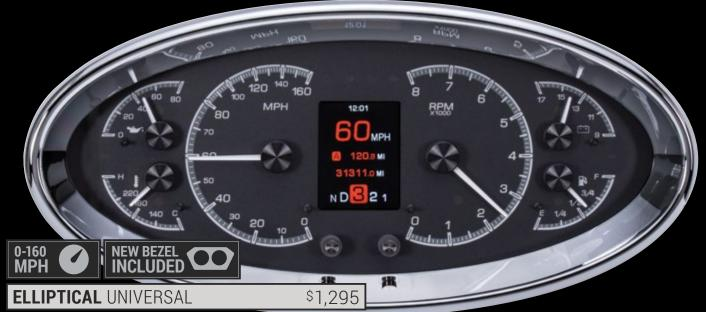
VHX and VFD3 options available. A chrome plated, billet aluminum front bezel with integrated rear housing makes this a one-piece solution. Six analog readings and a large  $\mathsf{TFT}$  message center are encompassed in the 12" x 5.75" body (11.75" x 5.3" cutout), which requires two inches of clearance on the backside. Built-in capacitive touch switches streamline installation, giving you the time you need to craft the perfect, one-off dashboard!
