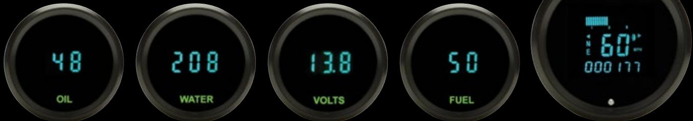
Complete five-gauge instrument package includes ODYR/SLX-01-6 speedometer/tachometer combo with a 3-3/8" housing, and the following with 2-1/16" housings: ODYR/SLX-03-1 oil pressure gauge, ODYR/SLX-04-1 water temp gauge, ODYR/SLX-05-1 voltmeter, ODYR/SLX-06-1 fuel level gauge. Includes: oil pressure, water temp, and speed senders (MPH/KPH selectable).
