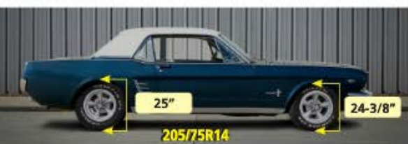
204/75R14 = fender lip is 24-3/8" front and 25" rear
