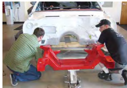
2. The new HEIDTS® Front Subframe and only four bolts, completes the installation to the body.
