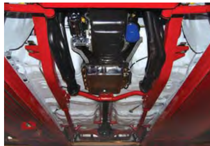
4. HEIDTS® Front Subframe with Subframe Connectors joins to HEIDTS® Rear 4-Link Kit.
