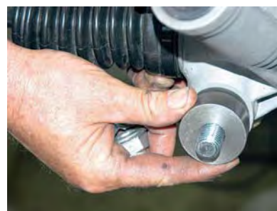
25) Before the rack-and-pinion can be installed, you have to install the bolts with a pair of spacers and washers.
