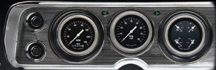
Dash bezel not included. Fuel sending unit not included, fuel gauge is calibrated to stock 0–30 ohms.
