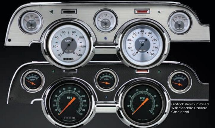
Fuel sending unit not included, fuel gauge is calibrated to stock 75–10 ohms.
