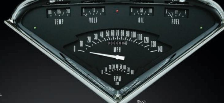
Fuel sending unit not included, fuel gauge is calibrated to stock 0–30 ohms.
