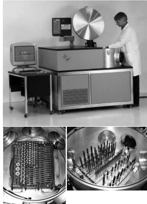
Figure 2. sp3 Model 600 Hot Filament Reactor with insert and round tool loads
