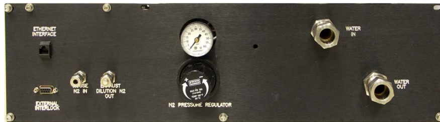
Facilities Panel located in the rear of the Reactor
