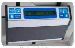
Optional factory-installed scale system
