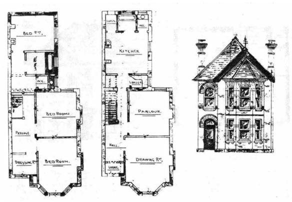
ABOVE:- FLOOR PLANS AND FRONT ELEVATION OF A WORKING CLASS HOUSE IN BOURNEMOUTH.
