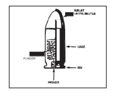
(Figure 3-1) Pistol Cartridge
