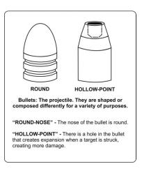
(Figure 3-4) Bullet (projectile) Design
