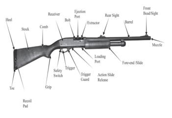
(Figure 2-5) Shotgun pump action nomenclature Position of parts may vary depending upon the make and model of the weapon.
