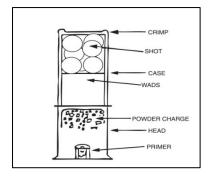
(Figure 3-3) Shotgun Cartridge
