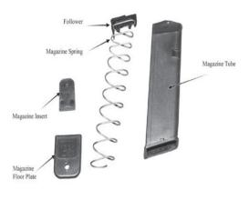
(Figure 2-3b) Semiautomatic pistol - magazine
