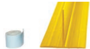
TC1279-570KIT Duct cable separator kit for 100mm, 220mm and 300mm duct The duct cable separator kit is installed longitudinally along the length of a duct run, to provide a separator or divider in the duct. The item is used to create separate compartments for different cords or cables.
