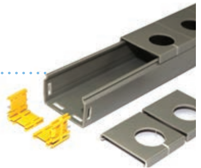
TC1279-570KIT Duct cable separator kit for 100mm, 220mm and 300mm duct The duct cable separator kit is installed longitudinally along the length of a duct run, to provide a separator or divider in the duct. The item is used to create separate compartments for different cords or cables.
