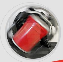
Gyroscopic mixing action turns containers end-over-end while simultaneously spinning.
