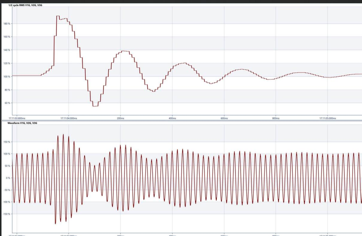
Graph displaying voltage swell in both RMS and Waveform value
