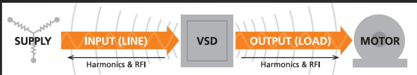
Harmonics in an electrical system can cause:
