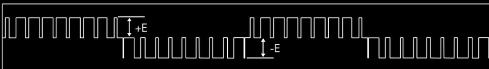
Line-to-line voltage waveform of 2-level PWM inverter
