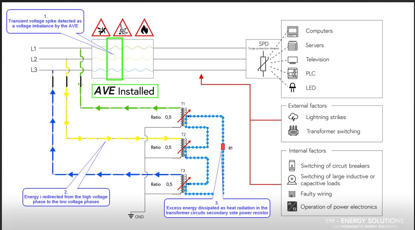
The figure visualises how the AVE mitigates transient voltage spikes
