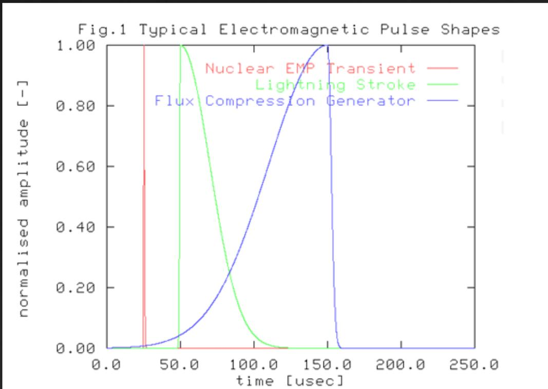
*Timespan and amplitude of EMP, lightning and flux compression transient event*
