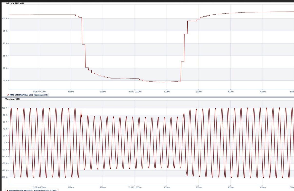
Graph displaying voltage sag in both RMS and Waveform value
