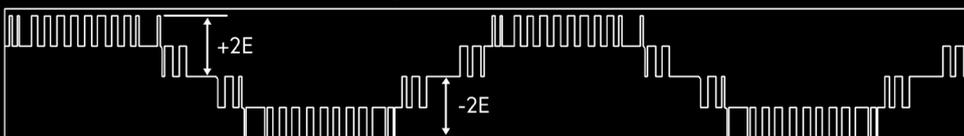
*Difference between 2-level and 3-level inverter technology*
