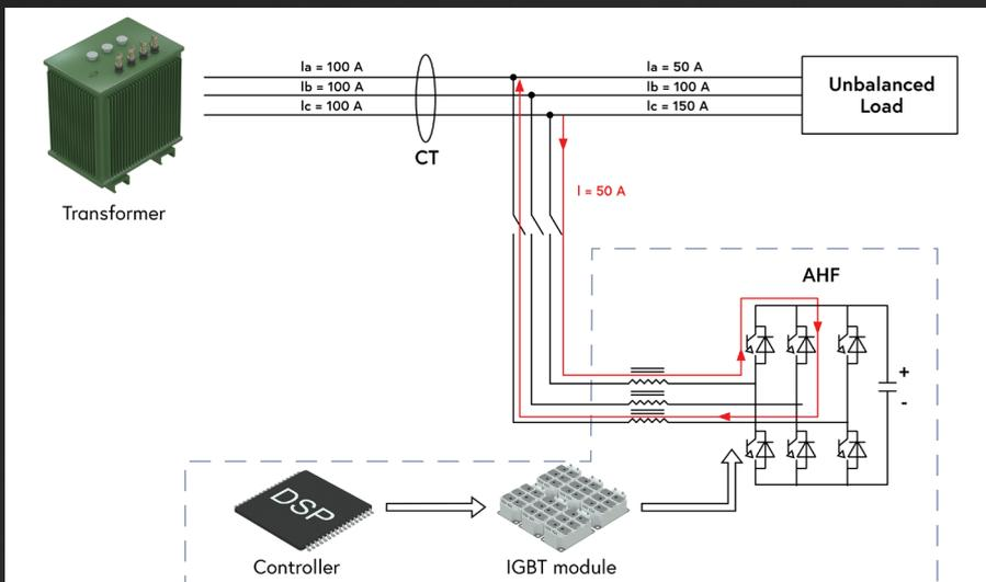
Load balancing principle SVG
