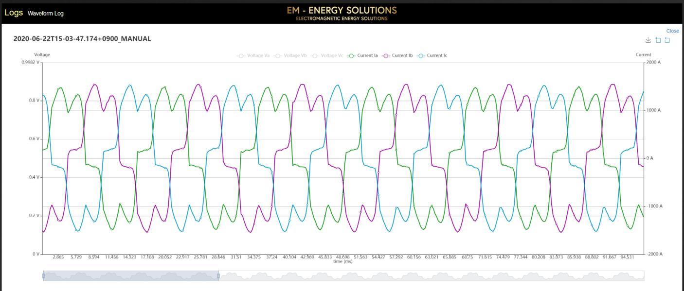
Current waveform distorted by 3rd (4%), 5th (29%), 7th (11%) and 11th (6%) current harmonics. THDi is at 34%, APF is not active
