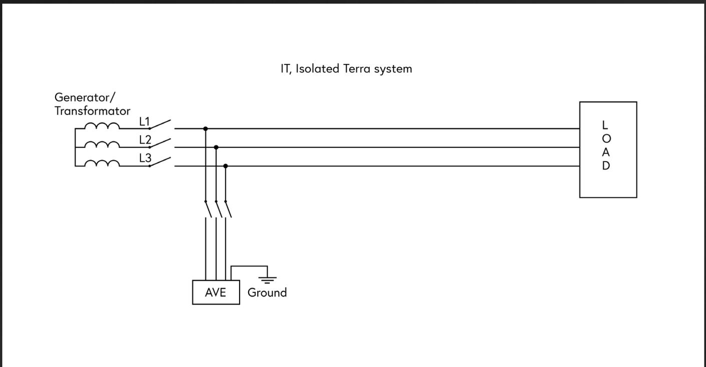
*AVE connects in parallel on distribution transformers secondary side*
