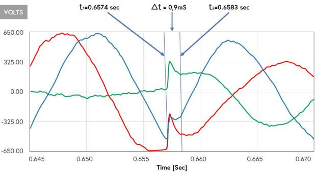
Loss of Phase (grounded) speed of operation
