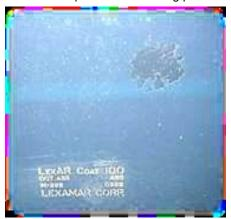
Here are the results of the initial sanding with 150-grit sandpaper. The darker spot is the acrylic starting to show under the clear coat.
