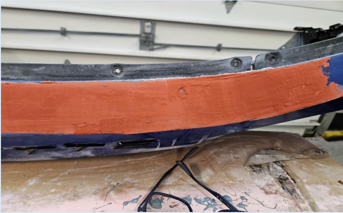
Damage caused by double-sided tape repaired with glazing putty.
