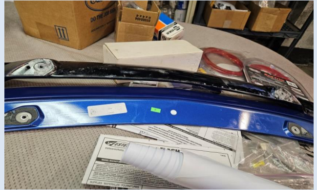
Comparison of OEM spoiler mounting holes to the aftermarket holes. Difference required me to drill two inner holes.
