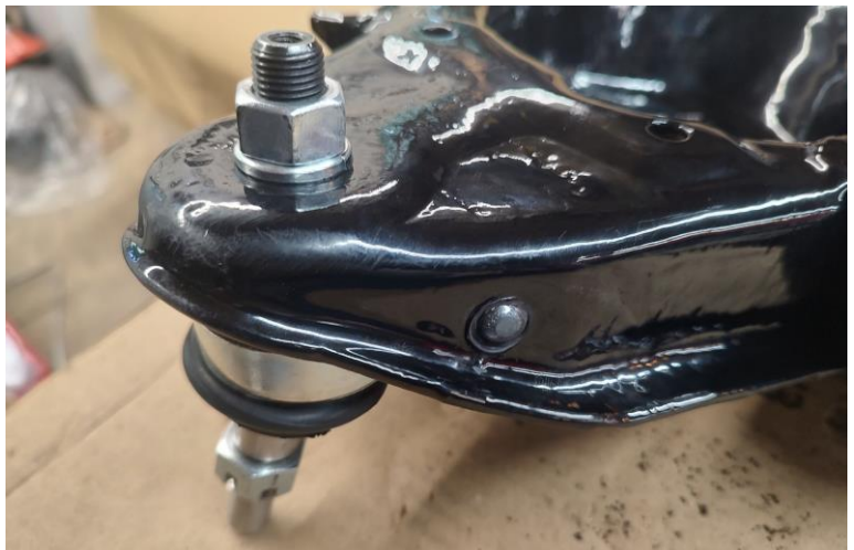
Figure 2. Note the rivet is painted black
