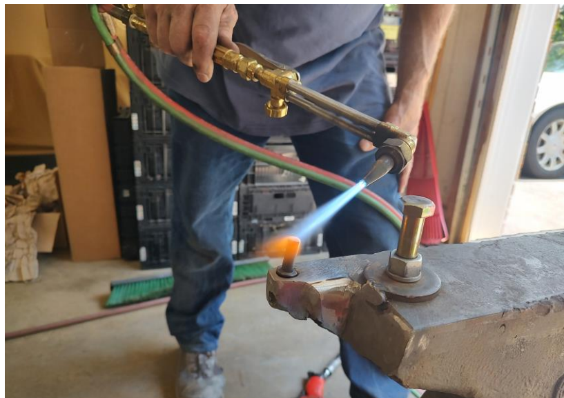
Figure 5 – Heating the rivet to get it “RED” hot!
