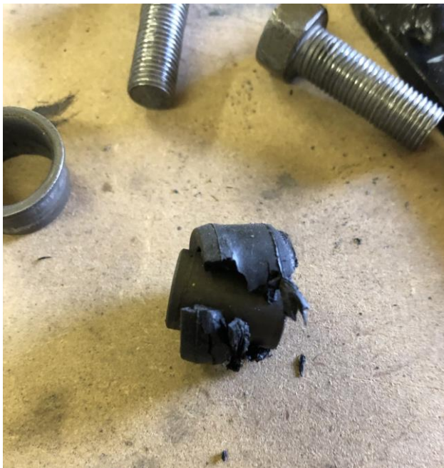
Disintegrated rubber bushing.
