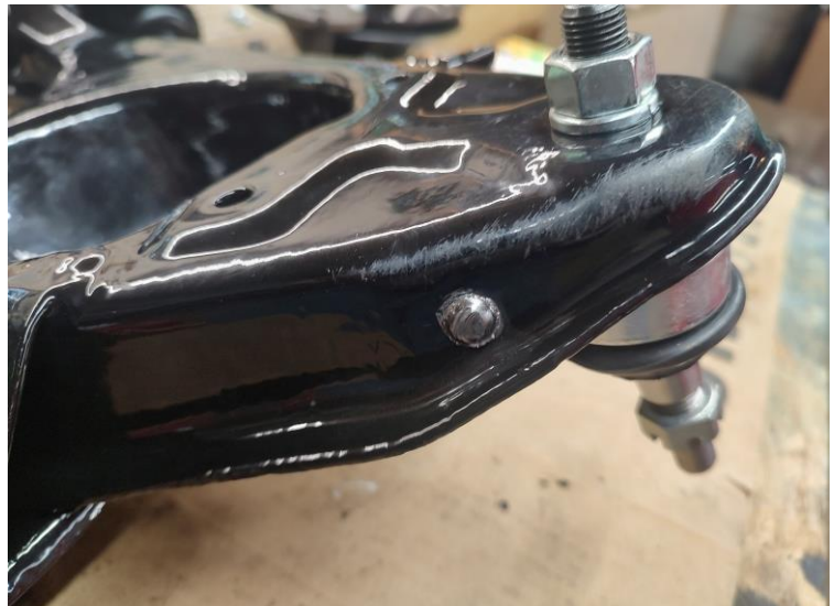
Figure 1 New rivet Installed
