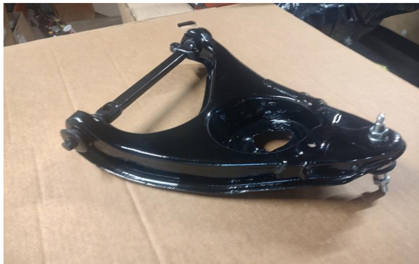
Figure 4 Note the unpainted ball joint
