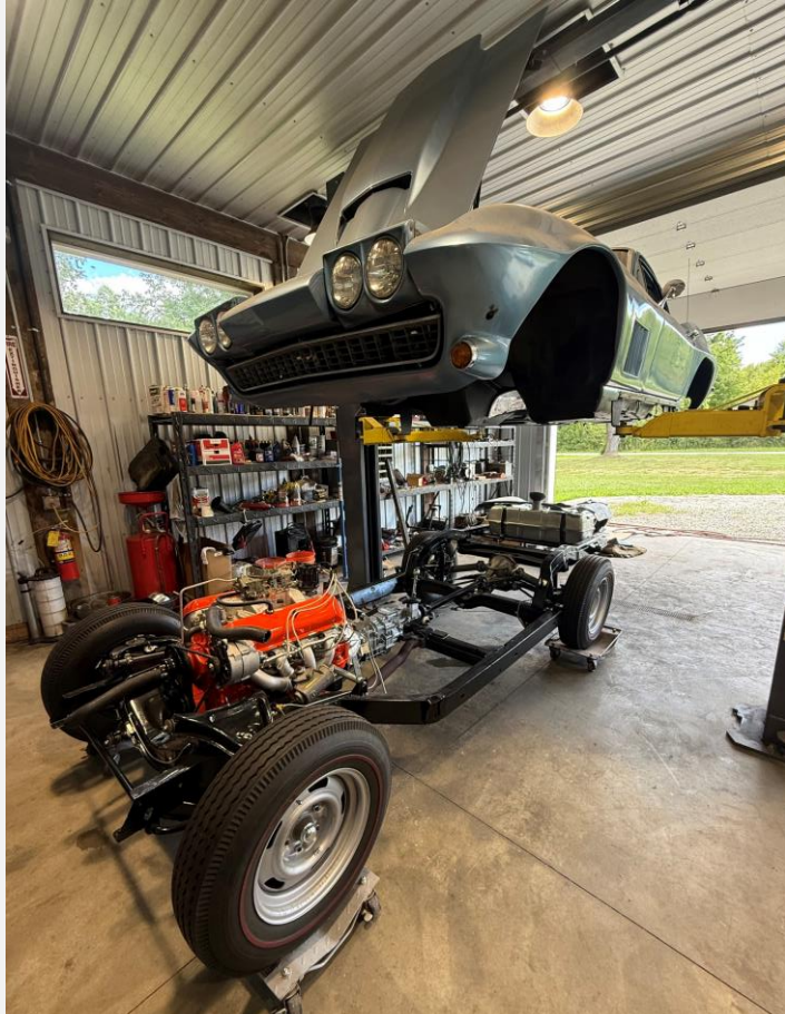
Restoration in progress-body lifted off the frame.
