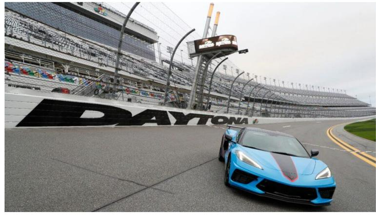
This mid-engine C8 Corvette Stingray coupe served as the pace car for the renowned Daytona 500 on Sunday, Feb. 14. At the heart of Corvette is a LT2 V-8, visible through the rear glass hatch, which produces 495 horsepower and 470 lb.-ft of torque when equipped with the Z51 performance package – the most horsepower and torque for any entry Corvette.
