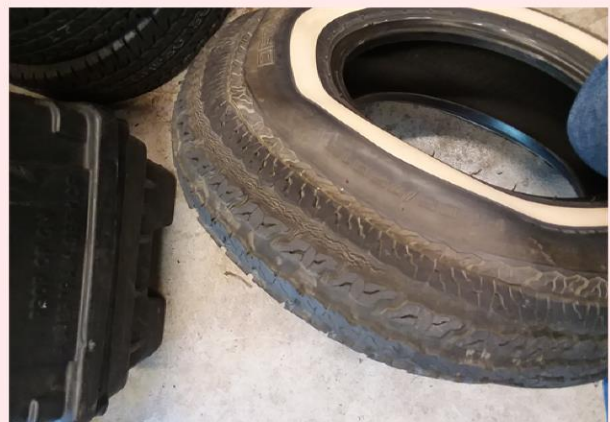
Side view showing bubble and dry rotting tire.
