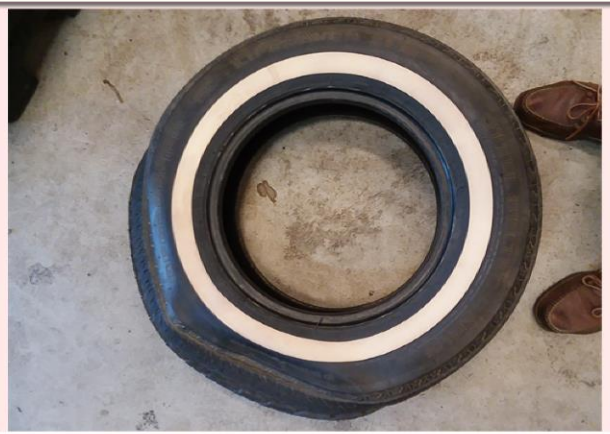
Side view showing bubble and dry rotting tire.
