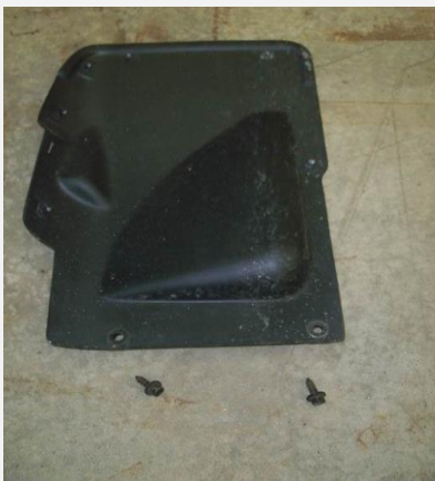
These two bolts attach to the metal triangular plate mounted to the fender.
