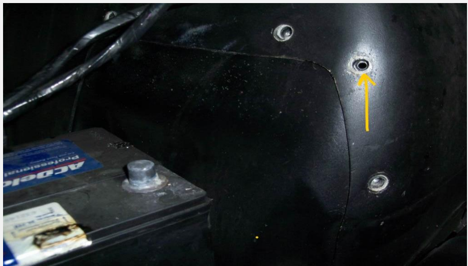
These two bolts attach to the metal triangular plate mounted to the fender.
