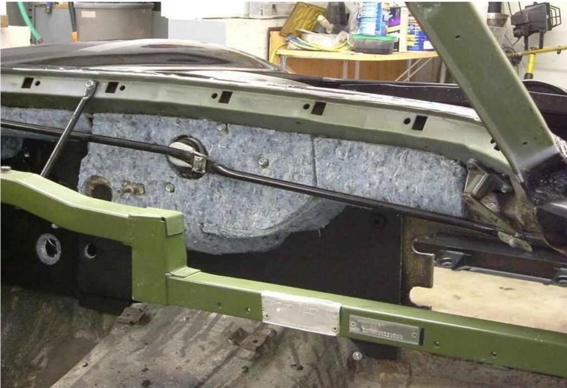
**Fig. 1 Wiper Arms inside the firewall.**
