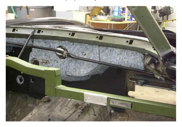
Fig. 1 Wiper Arms inside the firewall.
