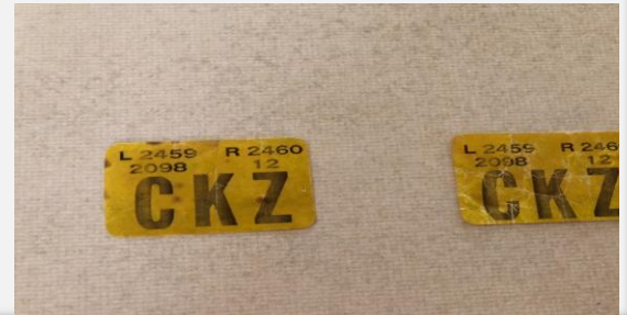
Fig. 9 – CKZ-Originals saved from a 1973 L82 Manual Trans. Found on both valve covers!
