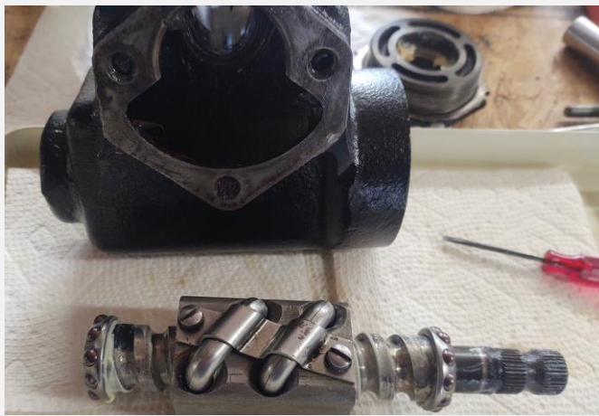
Fig. 5 Worm assembly all packed and ready for install.
