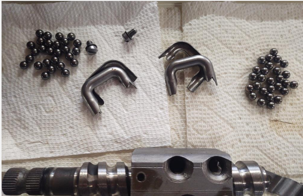
Fig. 4 -All 54 bearings accounted for! And ready to be packed in the worm gear.
