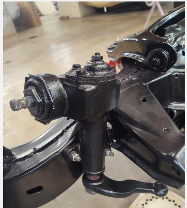
Fig. 6 Complete with a new gasket and installed on the frame and ready for relay rod and tie rod ends.
