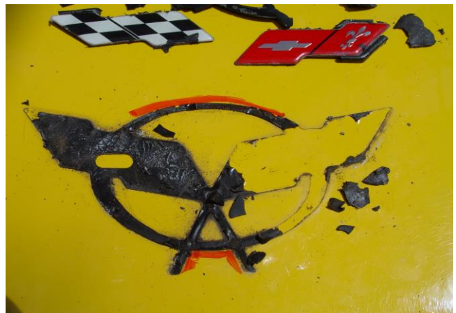
Fig. 2 Rear emblem removal. Note dry eraser positioning marks and original emblems pieces. To the left is adhesive that remains while right side removed.
