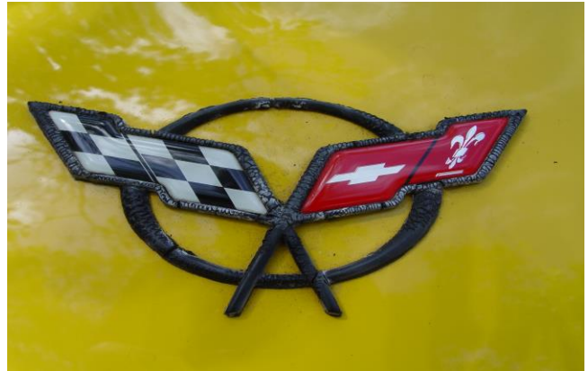
Fig. 1 C5 emblem. Note Cloisonné' intact but frame aged, cracked & deteriorated.
