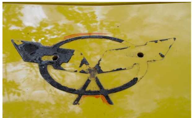
Fig. 3 Front emblem removal with holes for emblem positioning pins.
