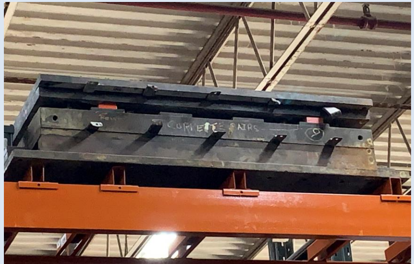
The mold for the front valance note: (Corvette-Bairs on front!)
