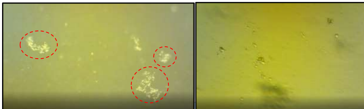
Figure 3.13. Floating sheets of translucent material in a wet sample as observed under an optical microscope. (b) The settled detrital material at the bottom of the slide. The shadows of the lighter floating material can be seen as dark hazy figures.
