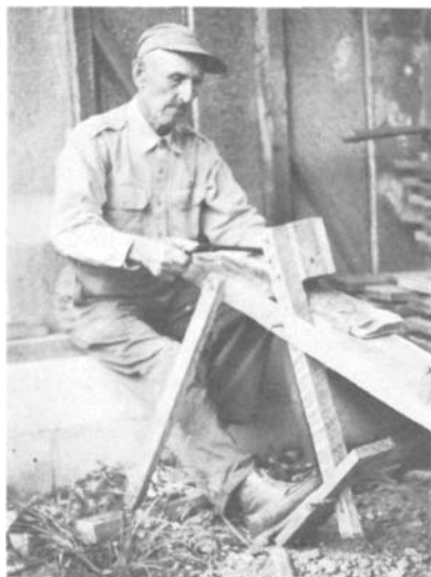
PLATE 38 Bill Lamb dressing a shingle with his shaving horse and drawing knife. As his foot pushes forward on the pedal, the block clamps the shingle in place.
