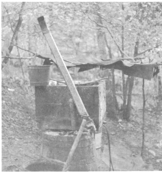
PLATE 274 The thump barrel and heater box. The drain pipe, when lowered, carries warm, fresh beer from the heater box to the cooker, the top of which is visible in the foreground.
