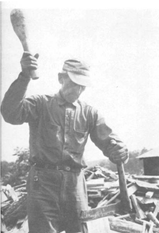
PLATE 28 The bolt now goes to the board "brake" to be converted into shingles. The brake, in this case, is the narrow "Y" crotch of a black gum tree cut about six feet long. The single end is propped up, and two stout poles are crossed in the double end. No nails or other braces are needed, for these poles wedge firmly enough to hold the end up. As one man said, "They work contrary to each other."
