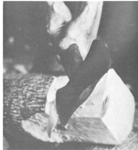
PLATE 65 Continue to hew until the top is smooth, and at the desired degree of slope.
