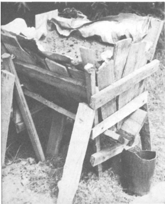
PLATE 215 A crude ash hopper, lined with paper and filled with hickory ashes, stands ready to work.
