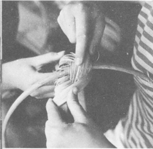
PLATE 173 When one split runs out, tuck in its end, insert the point of another into the weave, and continue.
