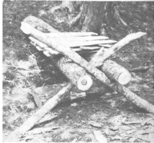
PLATE 28 The bolt now goes to the board "brake" to be converted into shingles. The brake, in this case, is the narrow "Y" crotch of a black gum tree cut about six feet long. The single end is propped up, and two stout poles are crossed in the double end. No nails or other braces are needed, for these poles wedge firmly enough to hold the end up. As one man said, "They work contrary to each other."
