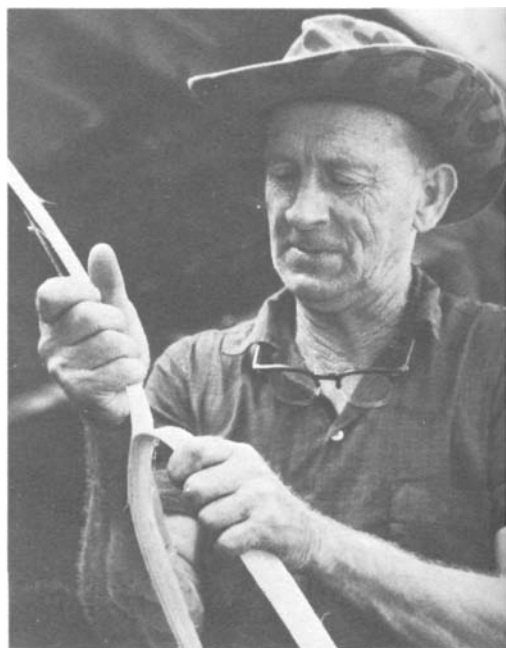
PLATE 157 If one edge binds or catches while the splits are being pulled apart, it can be freed using the knife.
