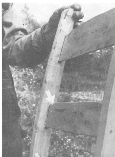
PLATE 189 The backs fit mugly into the slots just cut for them. Lon shapes the top corners (arrows) for decoration.
