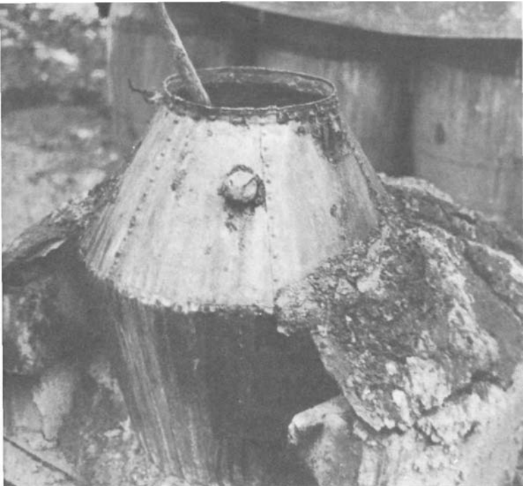
PLATE 273 The beer in this cooker is being heated prior to sealing on the cap. The swab stick resting in the cooker is used to stir the beer while it is heating to keep it from sticking to the sides and burning. Both this and the next three photographs were all taken at the same operation.
