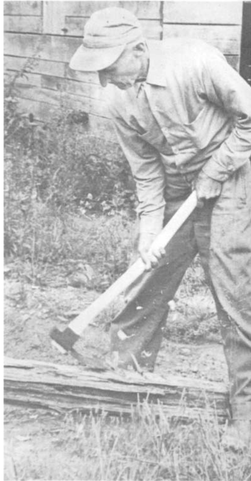
PLATE 17 The proper stance to use when working with a foot adze is demonstrated by Bill Lamb. The handle of the adze has a double curve for ease in working.
