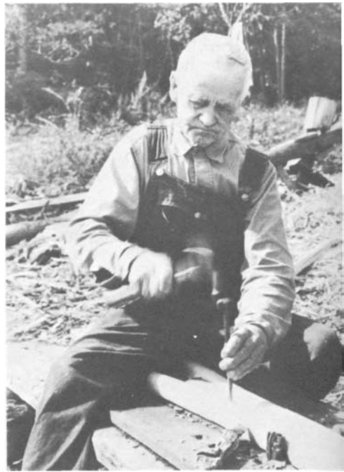
PLATE 186 A hammer and chisel are used to begin the slot that will hold one of the backs.
