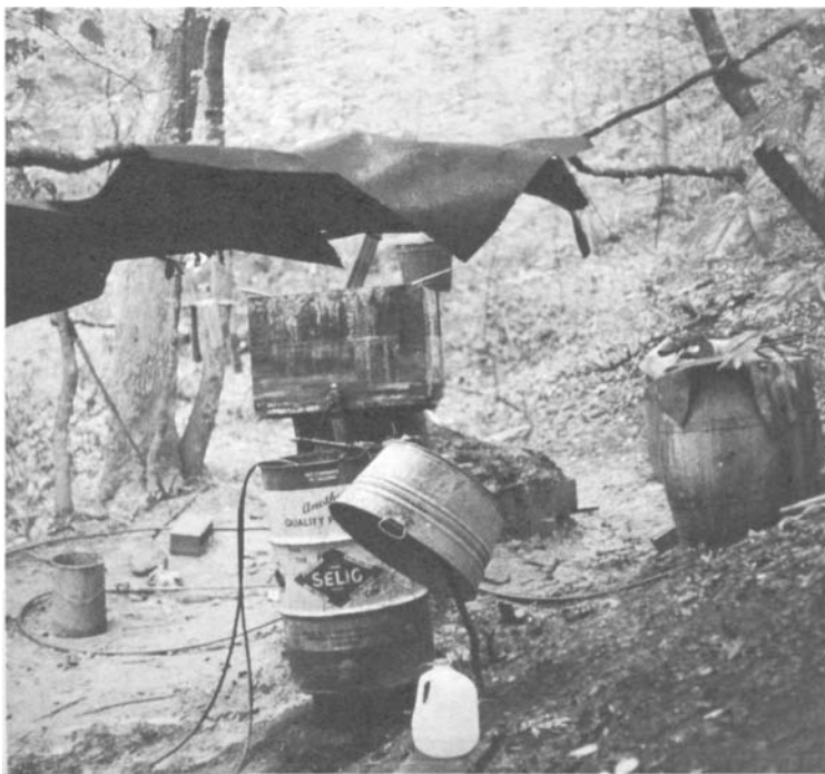
PLATE 276 The whole operation from the heater box, condenser end. The wooden barrels on the right are filled with fermenting mash. The furnace is hidden behind the heater box. The plastic gallon milk jar in the foreground is often used in place of glass jars for the finished product.
