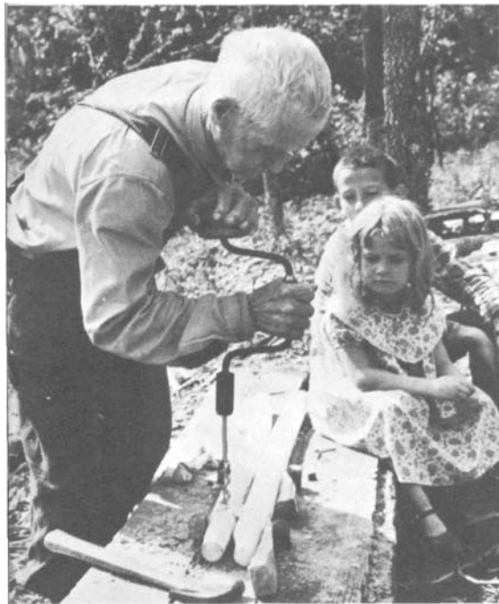
PLATE 185 Holes for the chair rounds are drilled while the legs are still pinned to the workbench.
