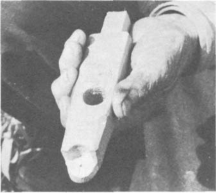
PLATE 192 This gauge helps shape the ends of the rounds in three ways. It . . .
