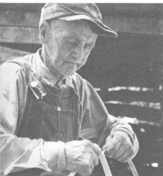
PLATE 156 Continue in this same fashion with each succeeding slice until the splits are the desired thickness.
