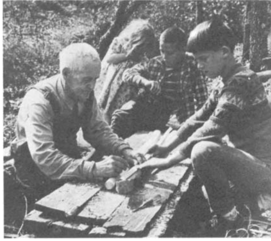
PLATE 184 With Donnie holding the measuring stick, Lon marks the locations for the rounds on each leg.
