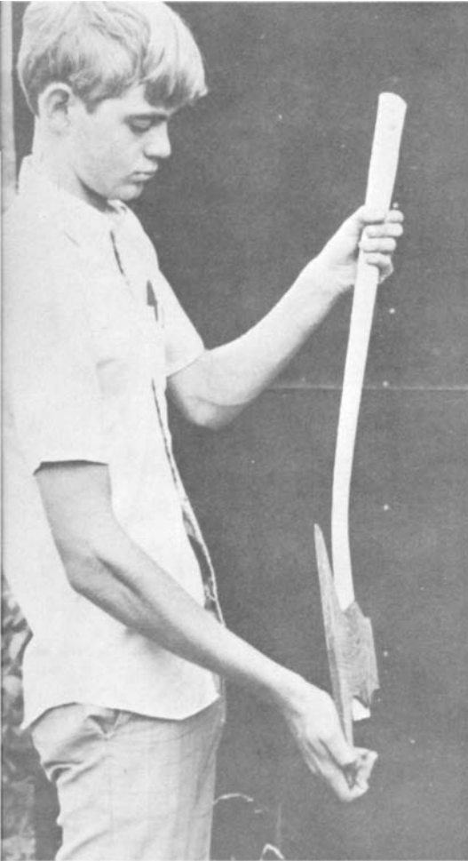
PLATE 16 As Paul Gillespie shows, a broadaxe has a curved handle to prevent the user's skinning his knuckles as he works.
