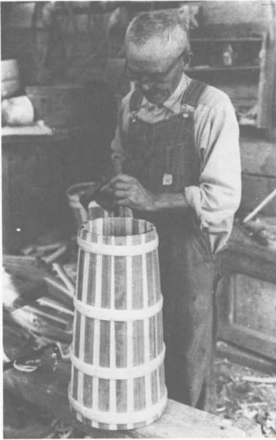
PLATE 388 Step 22: Add three more hoops, using the same procedure. With a handsaw, cut off the staves at top to even them. Use a rasp to smooth the top and bevel the edge.
