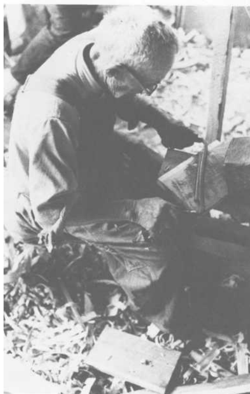
PLATE 359 Step 11: Use a shaving horse and drawing knife to smooth both pieces.
