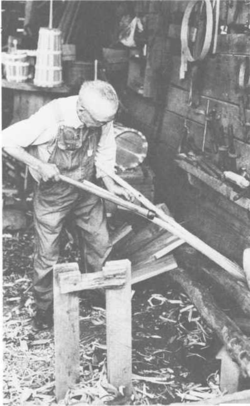
PLATE 372 Step 16: For the hoops, use green white oak. If the oak is dry, soak it overnight. Split the oak into strips using a froe and mallet. Measure the length with string, allowing six extra inches for the notch and lock.
