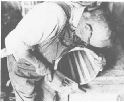
PLATE 353 Step 9: Use a croze (Plate 354) to cut a groove for the head to fit in.
