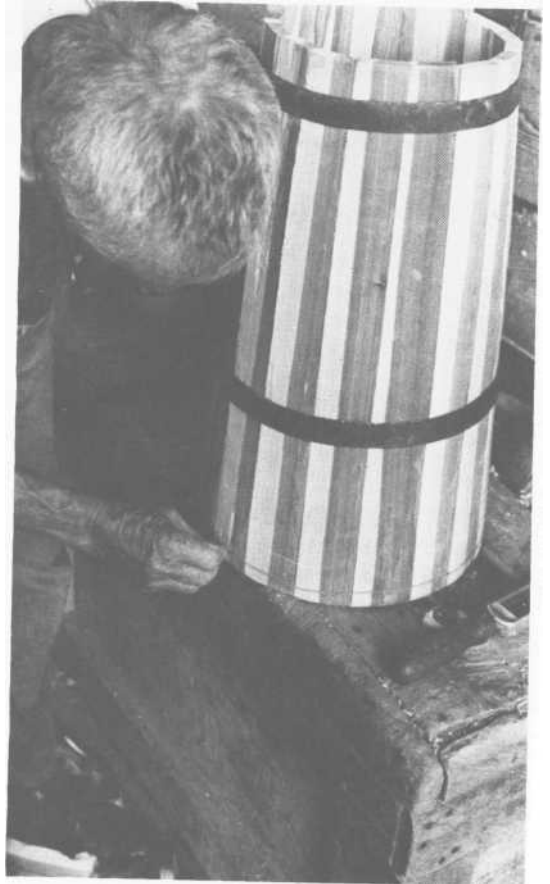
PLATE 371 Step 15: To measure for a permanent bottom hoop, take a string and measure the very bottom of the churn.
