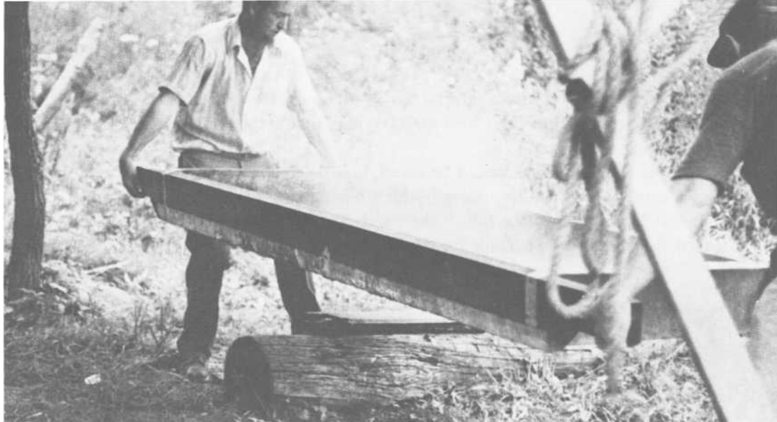
PLATES 428-430 The boiler-box is removed from the furnace ( Plate 428 ), and the sorghum is scraped down to one end of the boiler-box ( Plate 429 ). The sorghum is then dipped out of the boiler-box with a small saucepan ( Plate 430 ).
