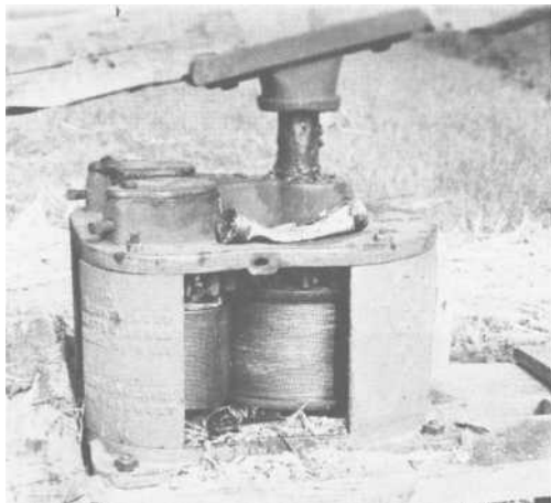
PLATE 415 Mr. Brooks's mill has three rollers (one is concealed in this photo).
