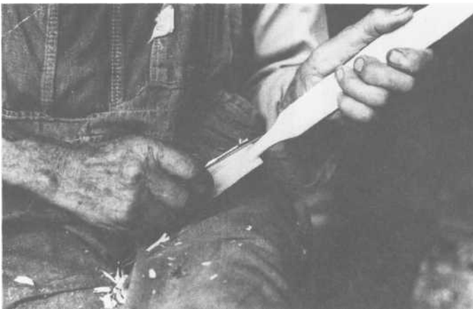
PLATES 379-381 On the opposite end of the hoop, cut with a knife as shown, until the inner side ( Plate 380 ) and the outer side ( Plate 381 ) are finished.
