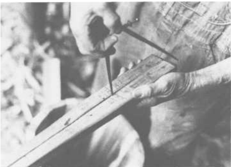
PLATE 339 Alex uses a compass to mark his gauge for different-sized churn heads.
