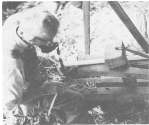
PLATE 373 Step 17: With a drawing knife and shaving horse, smooth the oak pieces to 1/8 to 1/4 inch thick and 1 to 1 1/4 inches wide.
