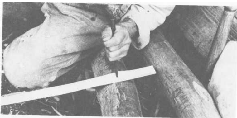
PLATE 376 To create the notch, place the chisel down on the hoop and hammer it through the hoop to make the first hole.
