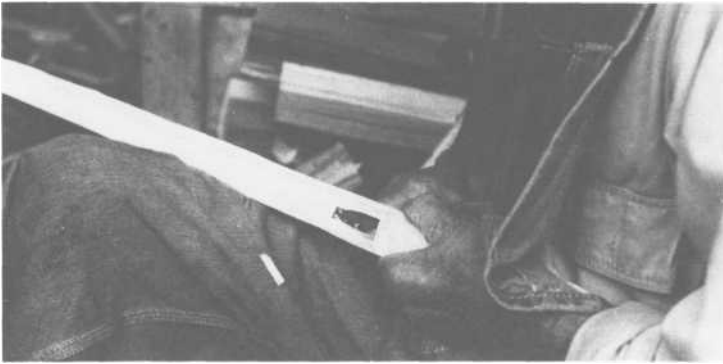
PLATE 378 Using a pocketknife, begin to cut out and shape the notch. Continue to shape the notch as shown.
