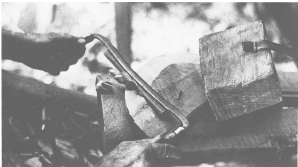
PLATE 364 Step 12: Begin to bevel the edges of the half-circles with a drawing knife.
