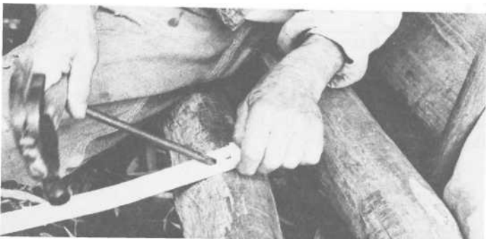
PLATE 377 Make a second hole with the chisel.
