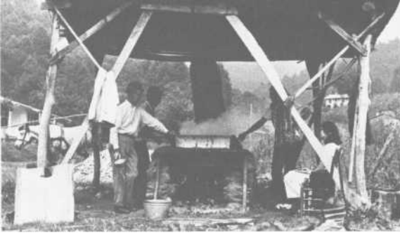
PLATE 424 The juice is brought to a boil. Some evaporators are slightly different than the Brooks's. Another example is shown as a diagram (Plate 425); numbers i through 6 indicate the sequence of the flow of the juice, number 7 refers to the boiler.
