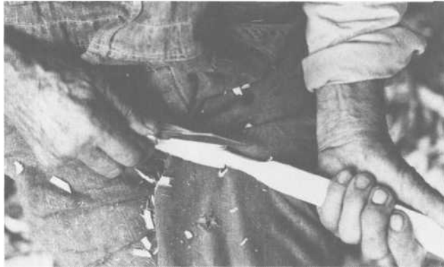
PLATES 379-381 On the opposite end of the hoop, cut with a knife as shown, until the inner side ( Plate 380 ) and the outer side ( Plate 381 ) are finished.
