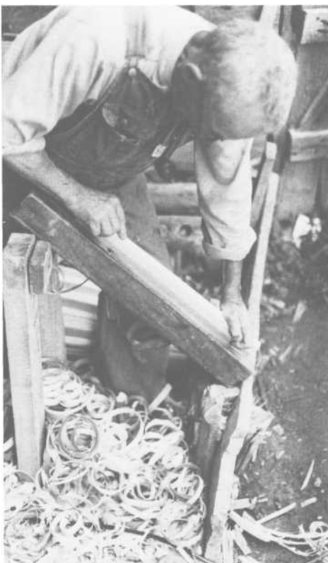
PLATE 340 Using a long-jointer, wood is planed from the edges of each stave until the angled edges fit the gauge.
