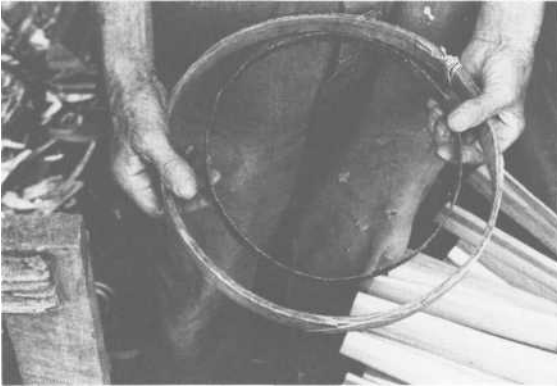
PLATE 343 Step 4: After staves are tapered and sides angled, Alex prepares to fit them into two temporary hoops.
