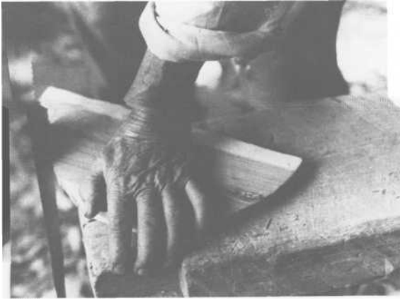
PLATE 361 Begin to cut the half-circles out with a handsaw. Saw as close to the edge of the half-circle as possible.
