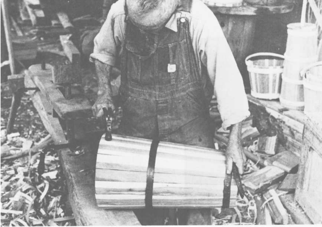
PLATE 368 Tap the staves with a hammer to make sure the head is in the groove tightly. Keep tightening the hoop with a chisel and hammer.
