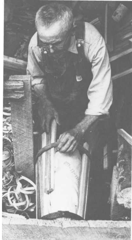
PLATE 346 The staves are added carefully.
