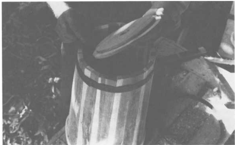
PLATE 389 Step 23: For the lid, obtain the circumference using the same procedure as for the head ( Plates'356—365 ). For groove on the underside of the lid, use a handsaw and trim with a pocketknife and rasp. Drill a hole slightly larger than the diameter of the dasher handle in the center.
