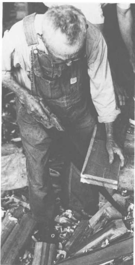
PLATE 358 For this churn, Alex used two pieces of board to make two half-circles.
