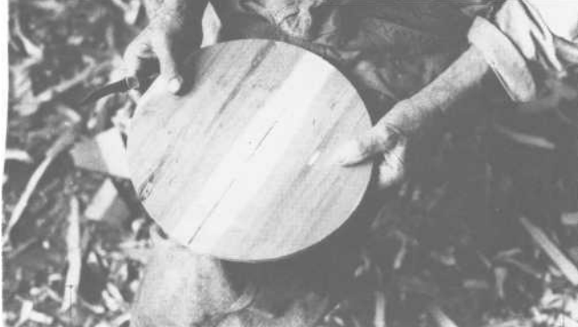
PLATE 363 After trimming, hold the half-circles together and check the smoothness of the circumference.
