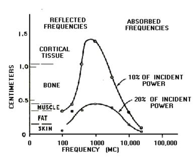
FIG 5 Microwave power distribution in the forehead model neglecting resonance effects and considering only first reflections (from Nieset et al (5), modified)
