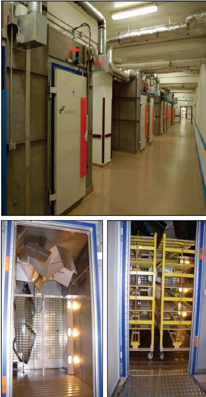
FIGURE 5 Exterior View of Chambers, Empty Chamber Showing the Vertical and Horizontal Stirrers, and Chamber with Cage Racks in Place
