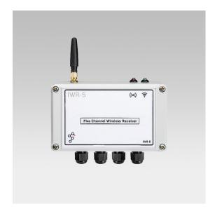
The IWR-5 is a five channel receiver designed to pair with the IWPT & IWTT wireless pressure & temperature transducers to form a cost effective replacement of the traditional wired transducers. This offers a low cost solution to inaccessible or expensive installation environments.
