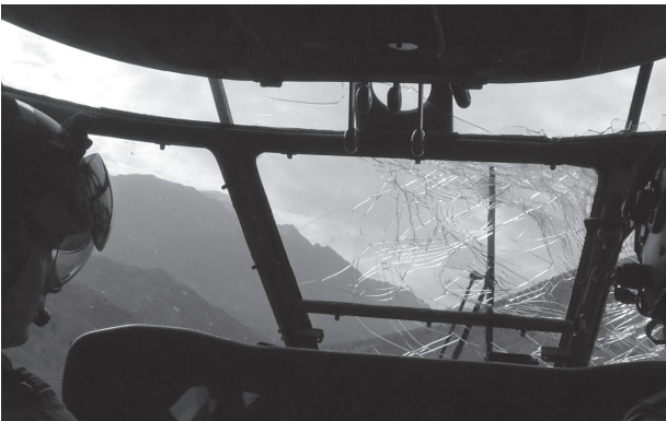
The view from the jump seat seconds after we hit high-tension electricity cables in Morocco
