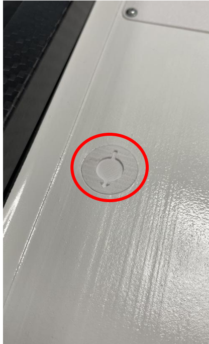
Figure 8 - Balance markers under the wing
