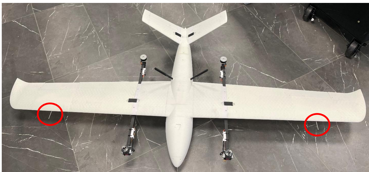
Figure 6 - Assembled UAS, with pitot probes highlighted
