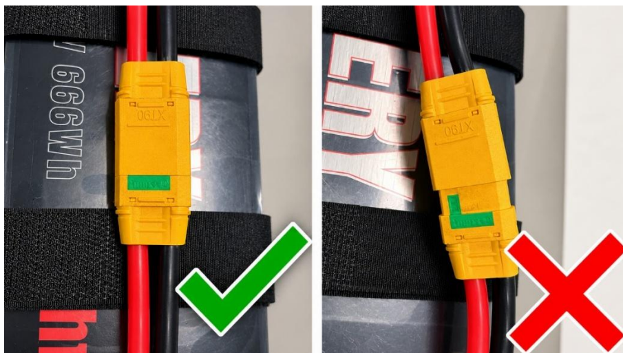
Figure 17 - Correct and incorrect way to connect the battery to the UAS
