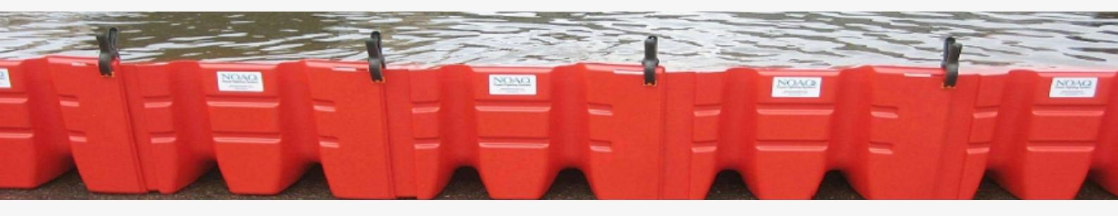
Each box consists of a damming part (the rear wall), an anchoring part (the horizontal section that rests on the ground) and a sealing part (the front edge of the horizontal section). Sealing strips of cellular plastic are fitted under the front and side edges. Each box is also fitted with three cellular rubber soles to create a good grip on the road.
