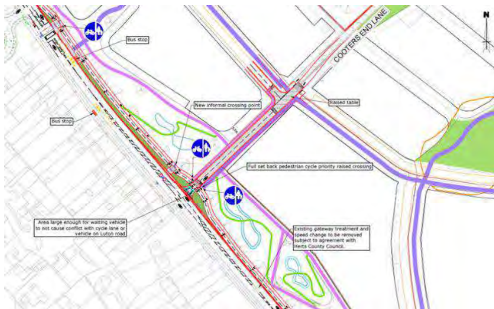
Figure 6: Drawing number 30984/AC/161 Rev B showing the proposed access junction on Cooters End Lane
