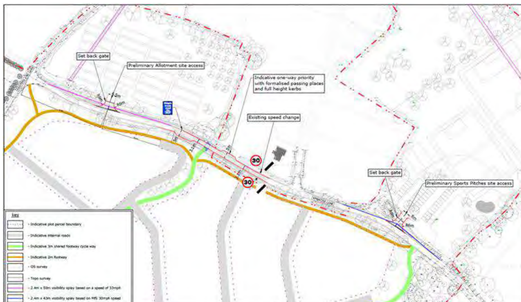
Figure 7: Drawing number 30984/AC/196 Rev A showing the proposed access junctions on Ambrose Lane
