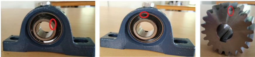
Fig. 2 Seeded defects of bearing and gear
