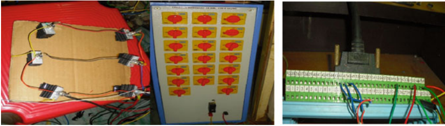
Fig. 4 Diode rectifier and PCI 1711/L Multifunction card
