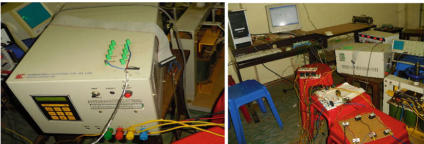
Fig. 5 Digivac inverter drive and experimental prototype
