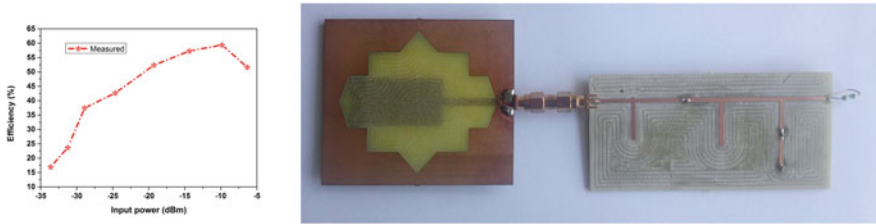
Fig. 10 Measured efficiency and fabricated prototype of the proposed dual-band rectenna
