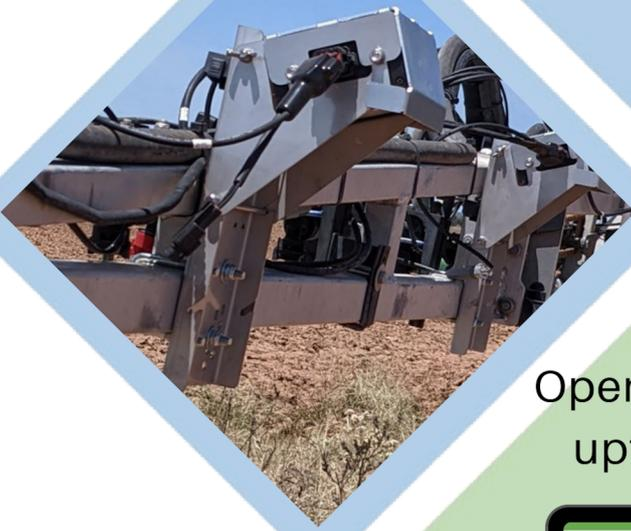
Easily remove cameras when not spot spraying
