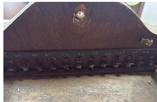
Connectors and switches at the top of the clock cabinet
