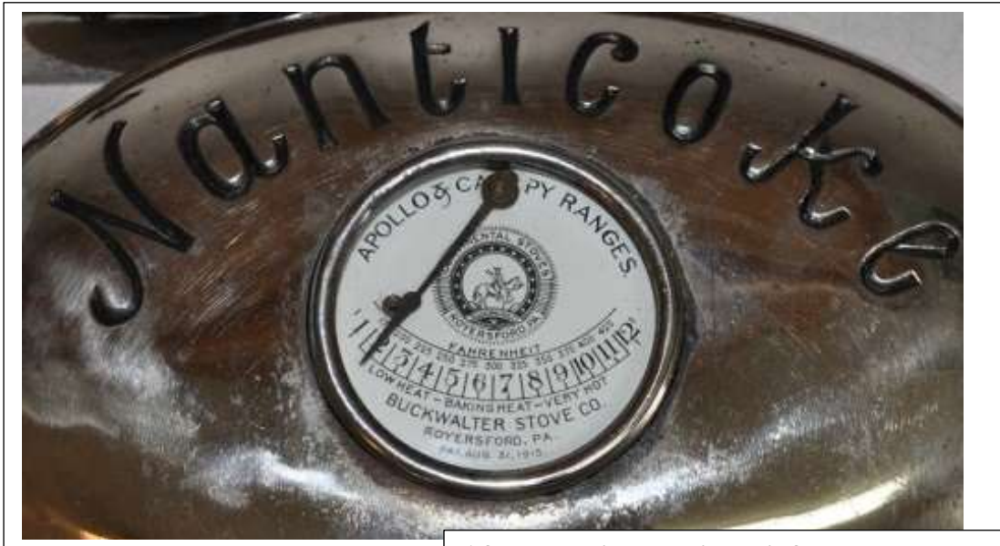
After extensive cleaning this face plate shows the temperature gauge and manufacturer, Buckwalter Stove Co. Pat. Aug 31, 1915.
